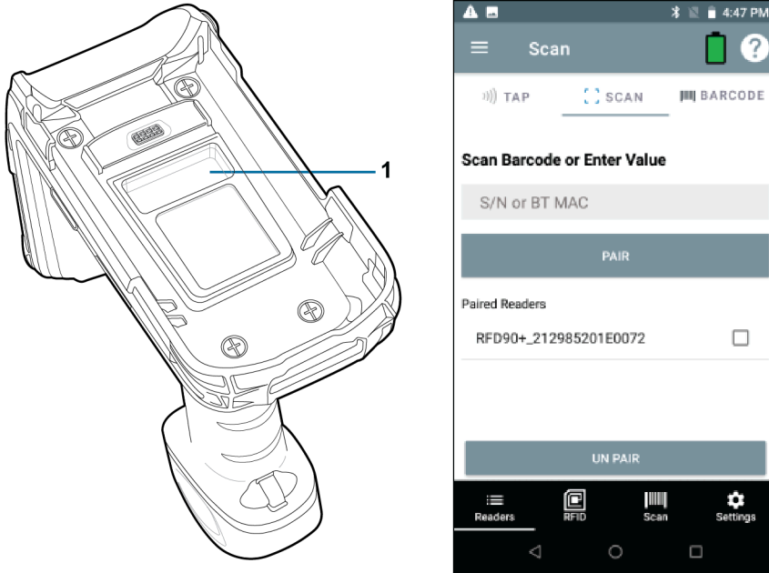
Figure 6 Scan 2D Barcode to Obtain MAC Address
